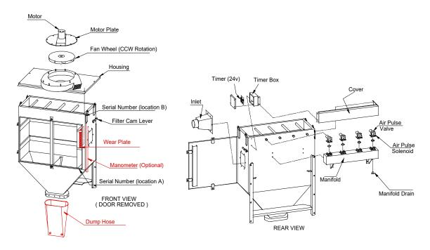
The dust collection cabinet has several components, which are important to the systems operation.
